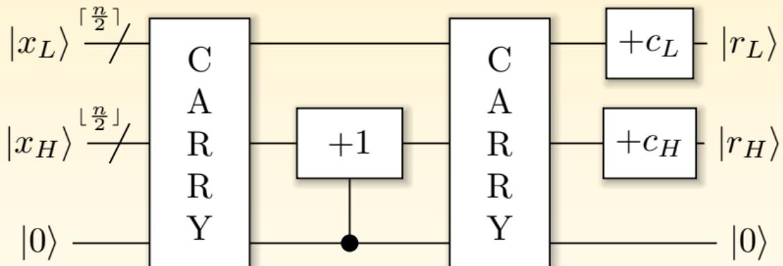
Note that this circuit uses a clean ancilla to detect if the final overflow happened.
